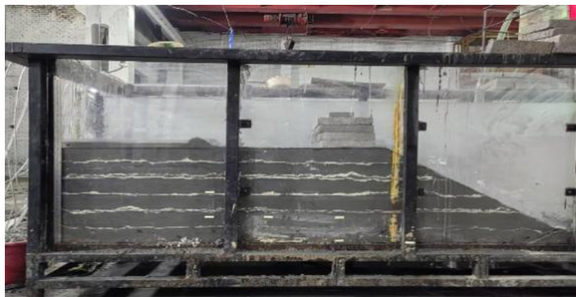
Figure 1. Schematic of lime layering and loading process.
