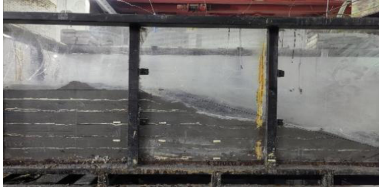
(b) Side view of tailings dam failure
