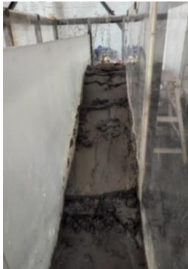
(a) Front view of tailings dam failure
